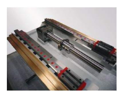
Both the transverse axis (X) and the longitudinal axis (Z) can be equipped with a brushless motor coupled with ball recirculating screws or with linear motors, controlled by optical linear scale. The support groups are built to use the system preferred by the customer.
